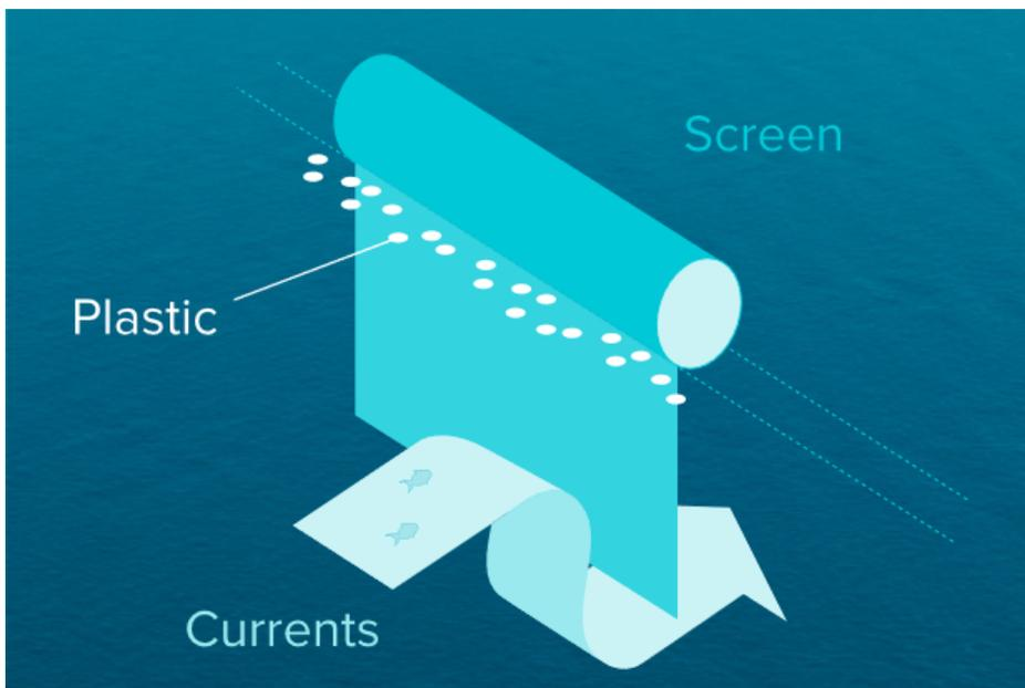
Figure 21.7. Diagram of plastic-catching screen deployed as part of the Ocean Clean Up project, to remove plastic from ocean gyres. From [www.theoceancleanup.com](http://www.theoceancleanup.com)
