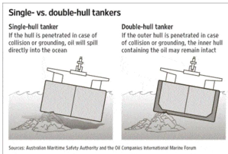
Figure 21.8. Double hulls on oil tankers are design to reduce the chance of an oil spill in the event of damage to the outer hull.
