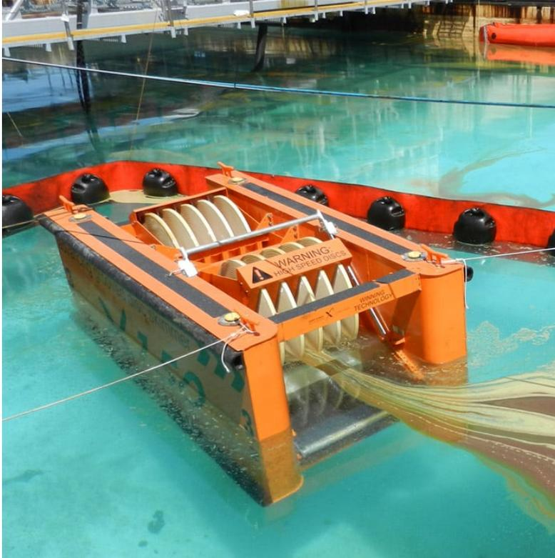
Figure 21.10. This skimmer is made with an oil-attracting material, which means oil adheres to the drum or disc and is separated from the water's surface. This type of selective skimmer recovers a high concentration of oil and very little water.
