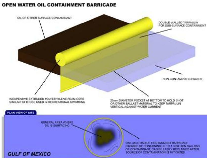
Figure 21.9. Oil-containment booms may be made of different materials (plastic, metal, oil-absorbent materials). The diagram here shows one possible type of boom, with a tarpaulin attached to a foam float.
